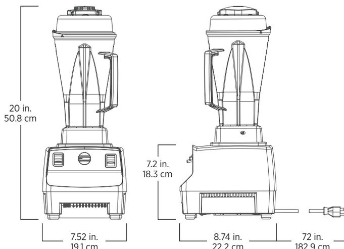
Includes Vita-Prep® with 64-ounce high-impact, clear standard container complete with Wet blade assembly and lid, tamper, and black base.
