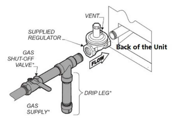
Prior to connecting the regulator, check the incoming line pressure. The regulator can only withstand a maximum pressure of ½ PSI (14" WC). If the line pressure is beyond this limit, a step down regulator before the regulator provided will be required. The arrow above (FLOW) shows gas flow direction and should point downstream to the equipment.
