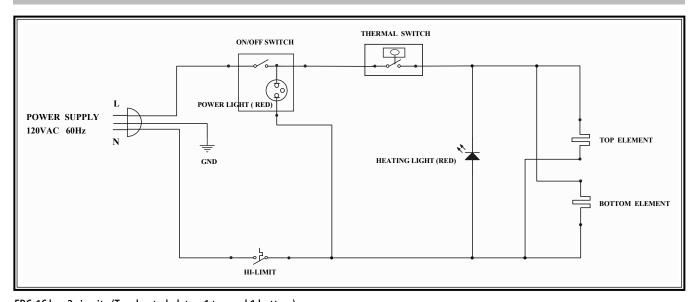
EPG-1C has 2 circuits (Two heated plates: 1 top and 1 bottom)
